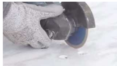
2. Cut with Diamond Blade Angle Grinder
