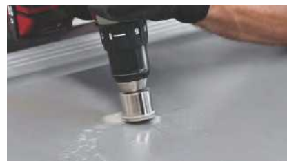
1. Round Cut with Diamond Blade Drill
